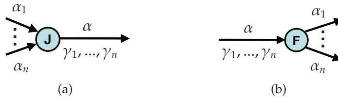
Fig. 43: (a) Join operator for merging n event streams into one structured event stream. (b) Fork operator for decomposing a structured event stream into n sub-streams.
