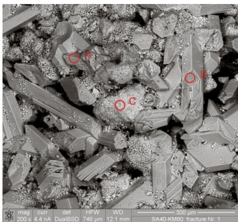
Figure 8-55: Point analyses of PT15 (SA40 KM60) fragment post free swelling test (cf. Table 8-12).
