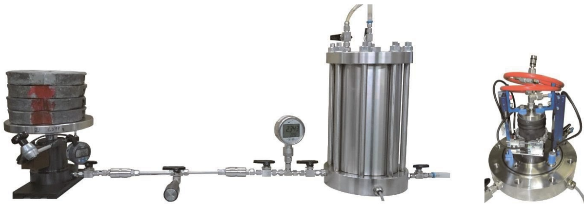
Figure 8-36: Isotropic compression tests: Photographs of the apparatus (left: isotropic compression cell from the outside, right: inside of the cell).
