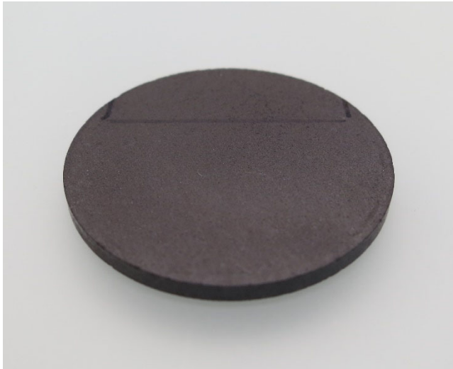
Solid disk from PANALYTICAL made of polycrystalline silicon. Its diameter is 3 cm
