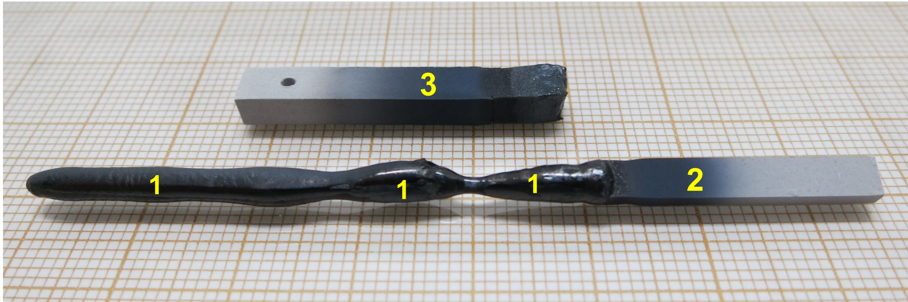
5 cm long as-grown crystalline material (1) plus polycrystalline seed rod (2) and remaining part of the polycrystalline feed rod (3)
