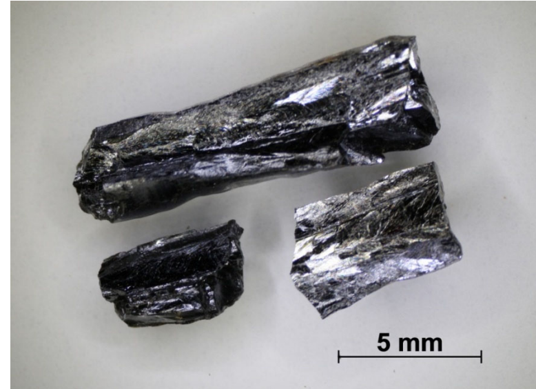
\text{La}_6\text{Ti}_4\text{Fe}_2\text{O}_{20} ( n = 6 ) Sample No. 523
