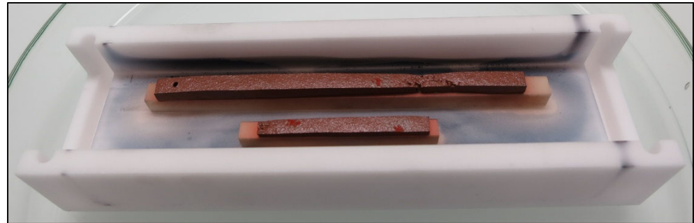
Rods with composition \text{NaWO}_{3.33} after they were heated and sintered under argon
