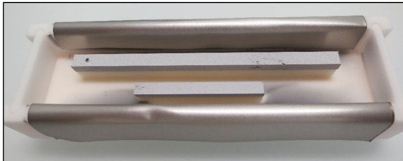
Two as-pressed rods with composition \text{NaWO}_{3.33}
