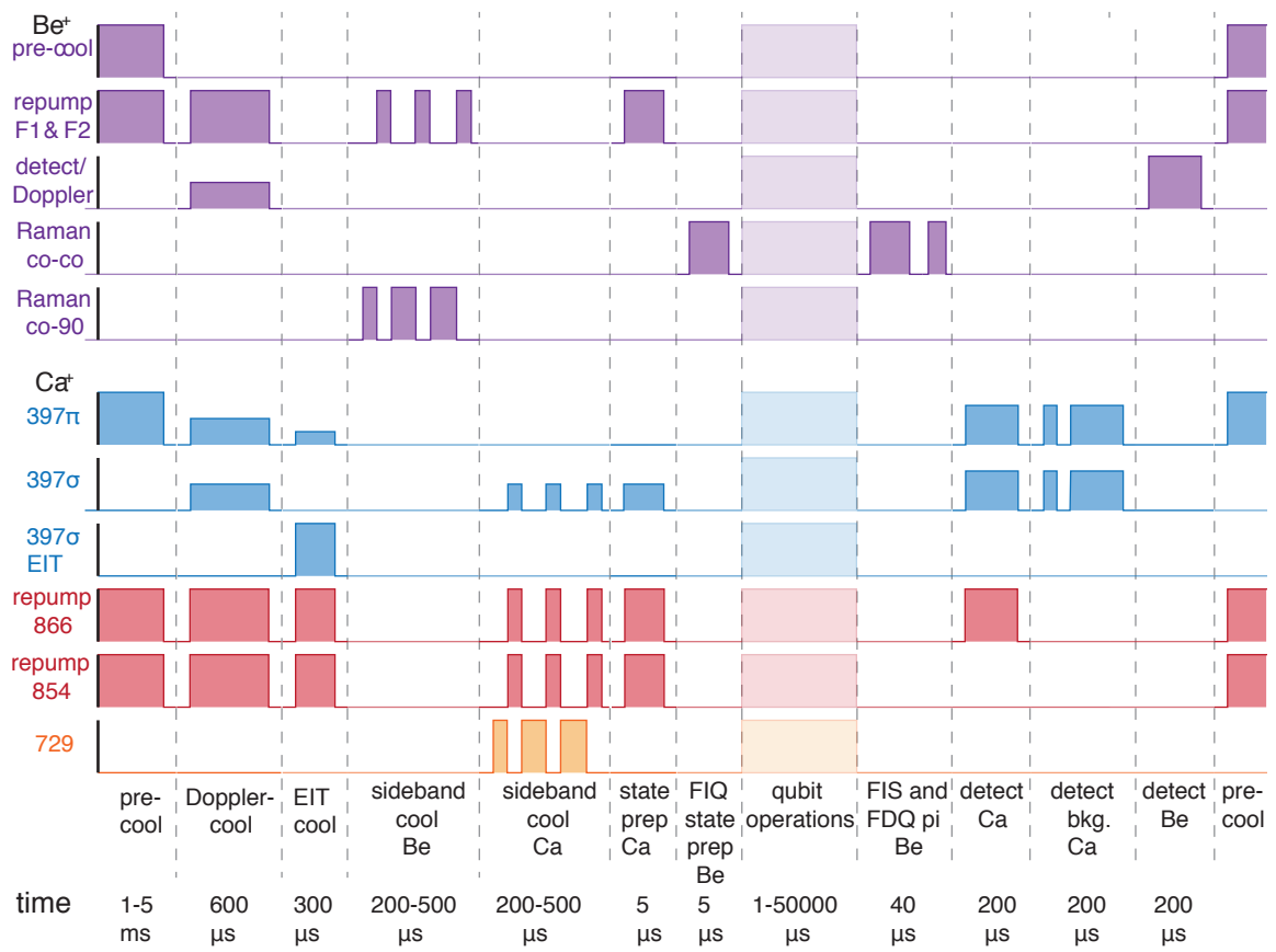
Figure 2.14: Pulse sequence diagram of a mixed-species experimental shot; At the bottom the typical length for each step of the sequence.
