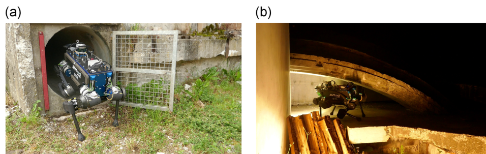
FIGURE 1 ANYmal autonomously navigating confined spaces using onboard mapping and no prior knowledge of the environment. The footholds, body poses, and transitions were all planned on the robot [Color figure can be viewed at wileyonlinelibrary.com ]
