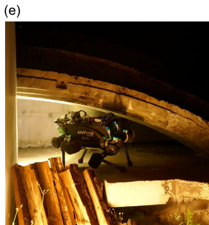
FIGURE 10 (Top) Rectangular Gap , (Middle) Crumbling Wall , and (Bottom) Collapsed Building . On the left are images of ANYmal completing each experiment, and on the right are corresponding plots of odometry. In the plots on the right, position is represented with solid, filled regions while rotation is represented with dashed lines. Within each plot, the top subplot shows roll, the middle subplot shows Y position and yaw, and the bottom subplot shows Z position and pitch. Shaded, colored regions represent the collision region of the widest part of ANYmal's torso. The dark gray regions are indicative of obstacles. Their heights are based on physical dimensions while their width represents the time between the front of the robot entering the confined space and the rear leaving [Color figure can be viewed at wileyonlinelibrary.com ]
