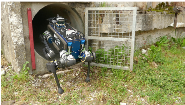
Figure 1: ANYmal autonomously navigating confined spaces using onboard mapping and no prior knowledge of the environment. The footholds, body poses and transitions were all planned on the robot.
