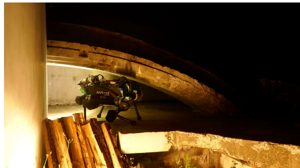
Figure 1: ANYmal autonomously navigating confined spaces using onboard mapping and no prior knowledge of the environment. The footholds, body poses and transitions were all planned on the robot.
