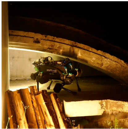
Figure 10: Top: Rectangular Gap . Middle: Crumbling Wall . Bottom: Collapsed Building . On the left are images of ANYmal completing each experiment, and on the right are corresponding plots of odometry. In the plots on the right, position is represented with solid, filled regions while rotation is represented with dashed lines. Within each plot, the top subplot shows roll, the middle subplot shows Y position and Yaw, and the bottom subplot shows Z position and Pitch. Shaded, colored regions represent the collision region of the widest part of ANYmal's torso. The dark gray regions are indicative of obstacles. Their heights are based on physical dimensions while their widths represents the time between the front of the robot entering the confined space and the rear leaving.
