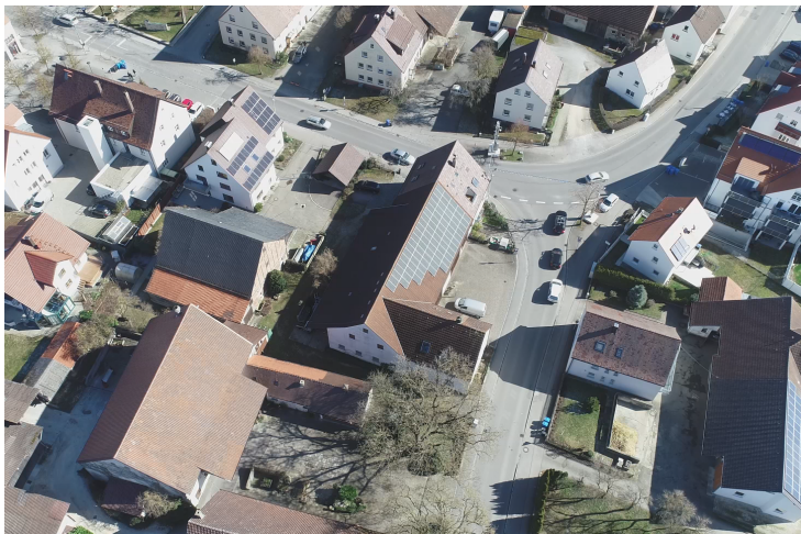
Figure 1.4: Drone footage of the MEC-View pilot intersection. Due to the long house at the intersection, approaching vehicles usually have to come to a stop at the yield line, before being able to observe the intersection.
