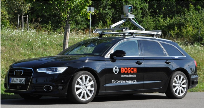
Figure 1.1: Automated Test Vehicle, equipped with multiple sensors. 360° surround view LiDAR mounted on the roof of the vehicle.
