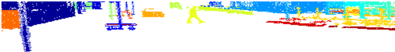
(b) Raw objects after ground plane removal and tracking. I.e. all objects that could not be associated for long-term tracking are removed as well. Each potential object is displayed with an individual colour.
