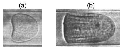
Figure 1. Pore flow of capsules with ovalbumine membrane: (a) parachute; (b) slug shape and folds in the azimuth direction.
