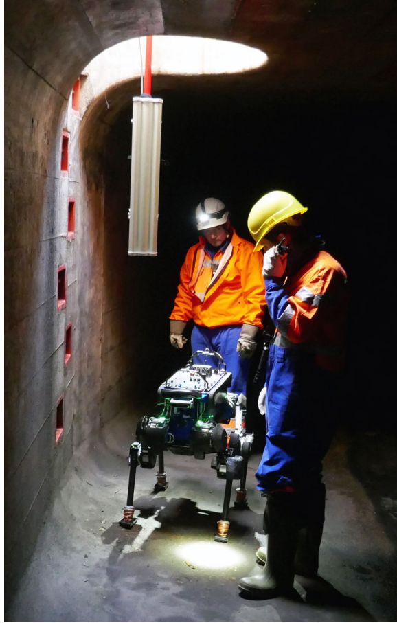
(a) ANYmal setup in the sewer
