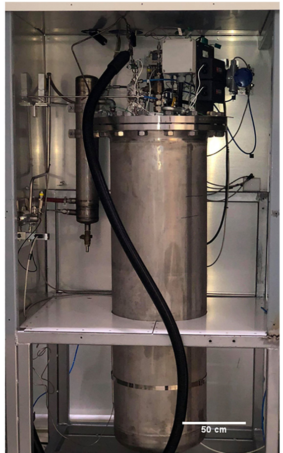
Fig. 4. The experimental setup [43,44,47] used for GSWS demonstration tests . a) schematic diagram, b) the actual reactor setup.
