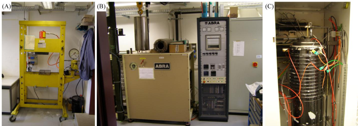
Figure 3.1: A) Hydraulic cold-press used during compaction stage 1. B) HIP machine, with extruded pressure vessel, casing and control panel, used for compaction stages 2 and 3a. C) Compaction stage 3b Paterson rig pressure vessel with cooling water tubes inside protective steel casing. This picture shows the machine set-up for a confined compression or furnace calibration test.
