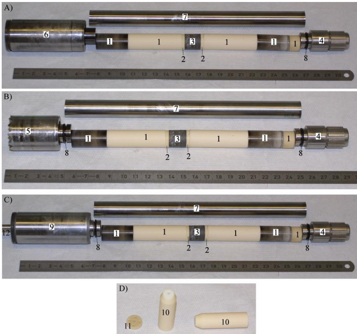
Figure 3.2A-D: Typical sample assemblies and parts for Paterson apparatus experiments in confined compression and isostatic stress mode (A), confined torsion mode (B) and confined compression or isostatic stress mode with imposed pore pressure (C). D Alumina rods used for 10 mm samples (10) and alumina spacer with five pore-pressure holes (11) used in pore pressure assembly.
