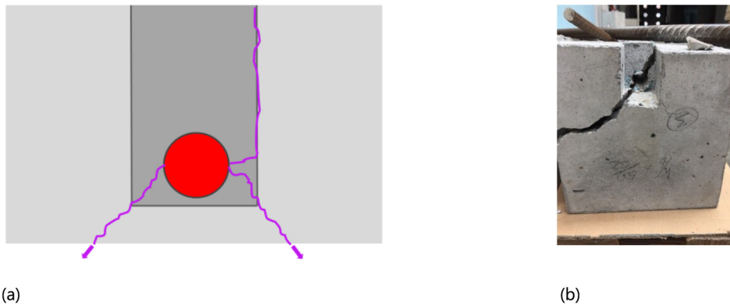
Fig. 15. (a) Illustration failure mode C and (b) example failure mode C.
