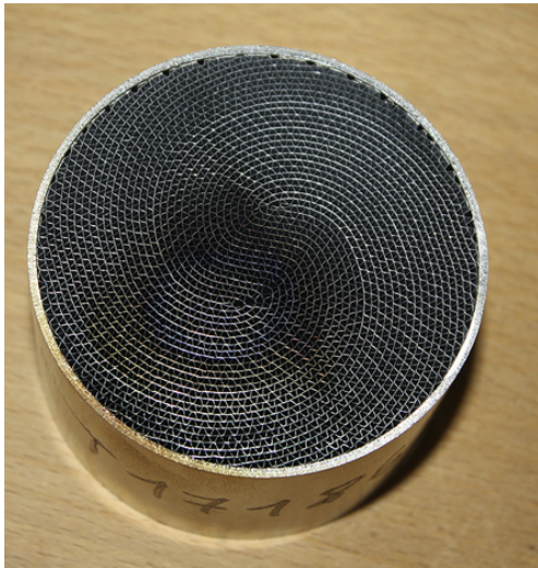
(a) Honeycomb structure made of an iron based alloy. This figure is copied from [28].
