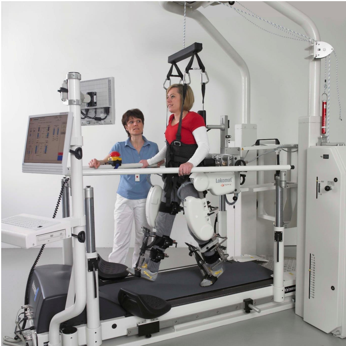
Figure 3.1: LokomatPro V5. The system is composed by a treadmill, a body weight support system, an orthosis with actuated hip and knee joints and force sensors and a display to show feedback to the patient. Picture: Hocoma, Switzerland.
