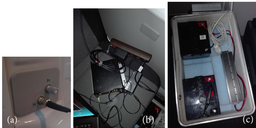
Figure D.1: Recovery material. (a) Antenna connection inside the recovery van; (b) portable receiver; (c) batteries.
