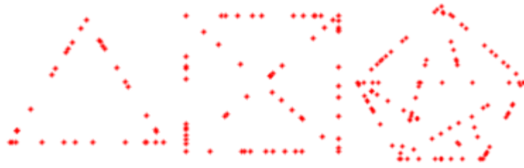
Figure 5-85. Edges and diagonals of a face are sampled with a random number generator which is initialized by the texture coordinates of the vertices of the edge or diagonal.
