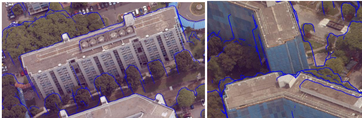
Figure 5-24. Boundary detection. Trees (left) and buildings (right) are highlighted by detecting the fracture lines in the geometrical map.
