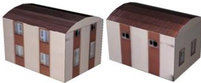
Figure 5-84. Building model with symmetries. Using a uniform sampling strategy will prevent ICP from recovering a rotation by 180^\circ
