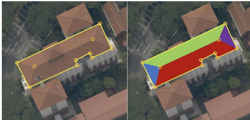
Figure 5-36. Illustration of multi-planes fitting algorithm. Left image: the keypoints are marked with yellow circles while the outmost boundary is marked with yellow polygon; right image: each fitted plane is filled with different color.
