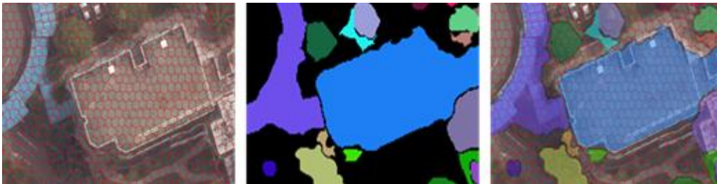
Figure 5-55. Assignment of side view features for each superpixel. From left to right, the images are the orthophoto with superpixels, above-ground segmentation (colour blocks) and their overlap.
