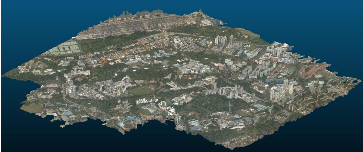
Figure 5-6. Dense point cloud of the NUS campus generated from 306 vertical and oblique images of the 5-head camera by Pix4D Mapper.
