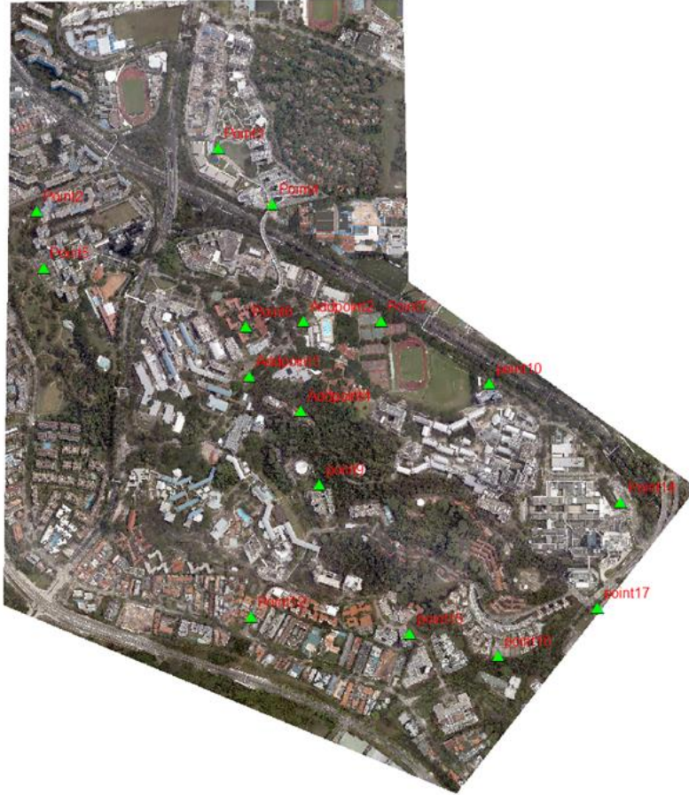
Figure 5-1. Distribution of the GCPs. The locations of the GCPs are marked with the green triangles and the names are in red. Area size ca. 2.2 sqkm
