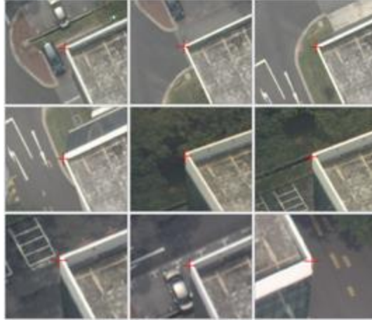
Figure 5-20. The estimated image coordinates of a keypoint (the roof's corner) in all images.
