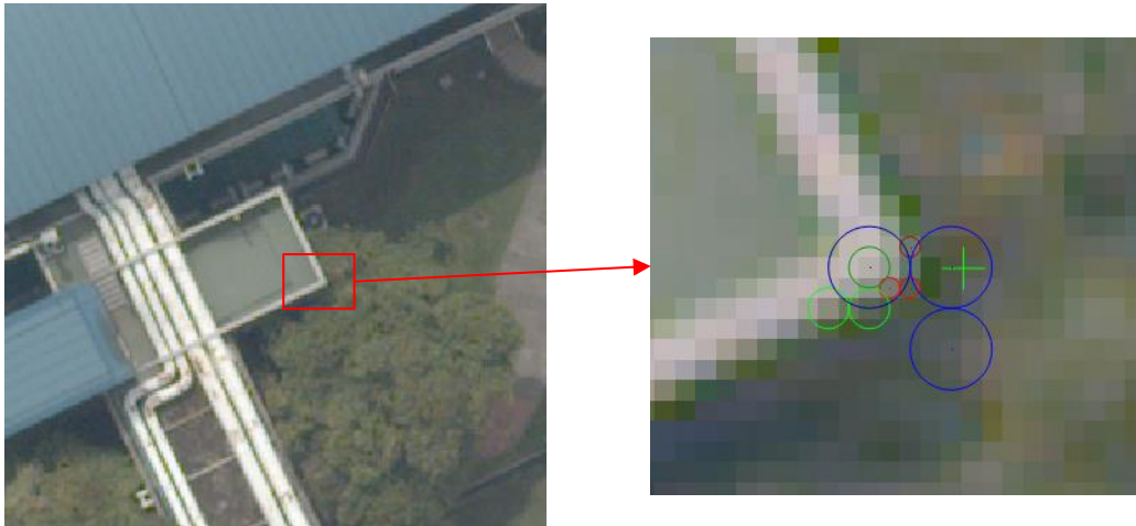
Figure 5-17. Harris detection for the double-edge corner. Nine candidate points from three levels of the image pyramid are detected and marked by different kinds of circles in the image. The size and the color of the circle imply which level the point comes from. Three red circles are Harris points from the original image level, three green ones are from the middle level and the three blue ones are from the top level.
