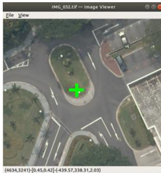
Figure 5-26. Street lamp in the top view, the green cross is the keypoint detected by the Harris detector.
