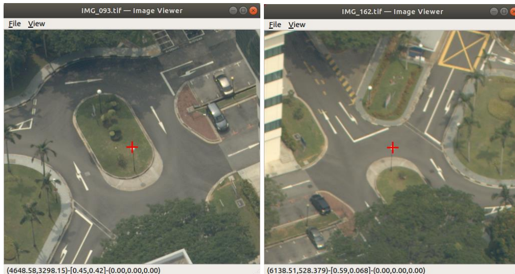
Figure 5-28. Point locations after applying the epipolar-line based multi-view matching.
