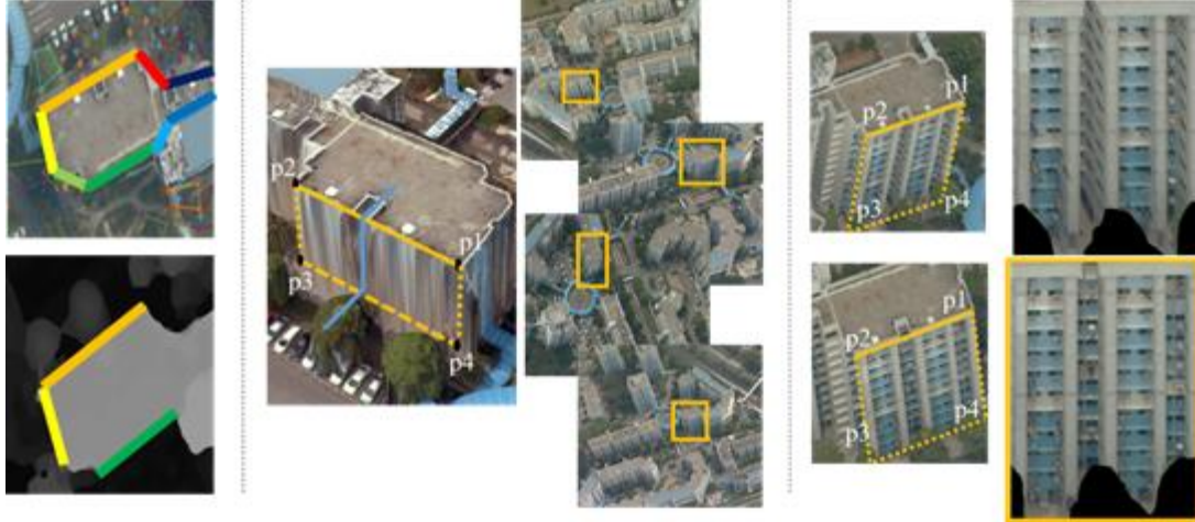
Figure 5-53. The side view texture extraction from multi-view oblique images. From left to right, the images are the polygon boundaries, the 3D vertical face and its projections at the oblique images, and the side view textures with a rectification. More details are explained in the text.
