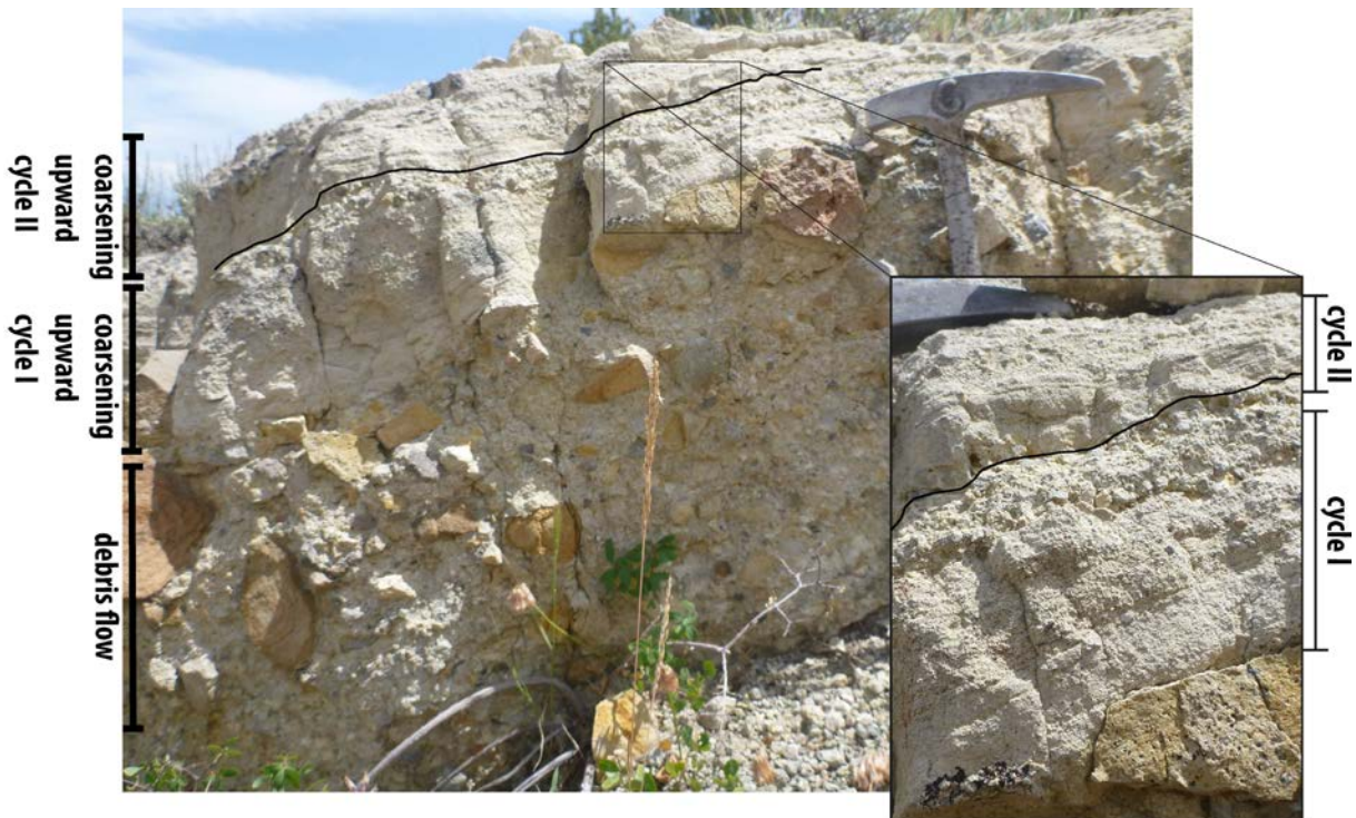
Fig. 3 Coarsening upward cycles in ash layers overlying debris flow deposits. The bedding is clearly recognizable and dips with 20° towards SE. The text for general composition of debris flows. (Location on geological map RCX6_4
