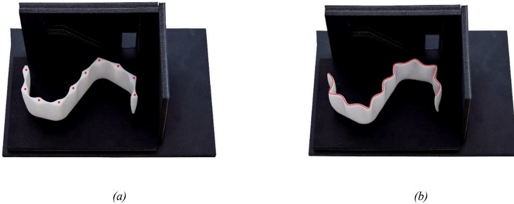
Fig. 19: Design examples for different structural scenarios: (a) local thickening of the wall as a reaction to concentrated loads; (b) local undulations as a reaction to linear loads.
