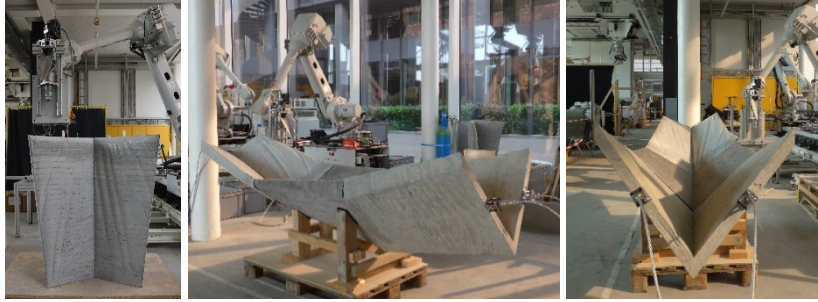
Figure 9. Prototype (foil formwork) and post-tensioned folded roof section
