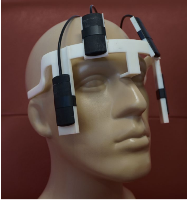
Figure 2.3: Four NMR markers were attached to a 3D-printed headset. The support points of the headset are above the ears and between the eyebrows on the nasion.
