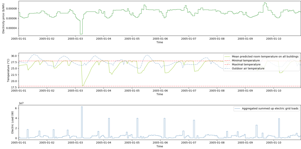
Figure A4 Room temperatures and energy loads on all buildings of the district in our model during the first ten days of January 2005 in Singapore, with price-based demand flexibility
