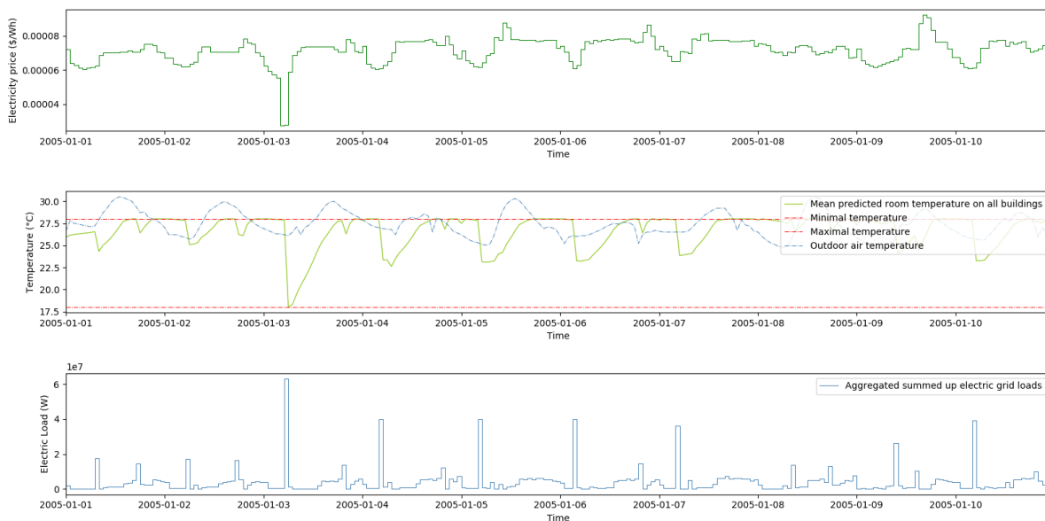
Figure 1 Room temperatures and energy loads on all buildings of the district in our model during the first ten days of January 2005 in Singapore, with price-based demand flexibility
