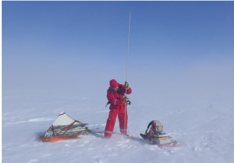
Fig. 7. Accumulation probe measurements for the detection of hard layers in the subsurface. One 90 cm corner reflector is visible on the sledge on the left as well as the GPR system on the right.
