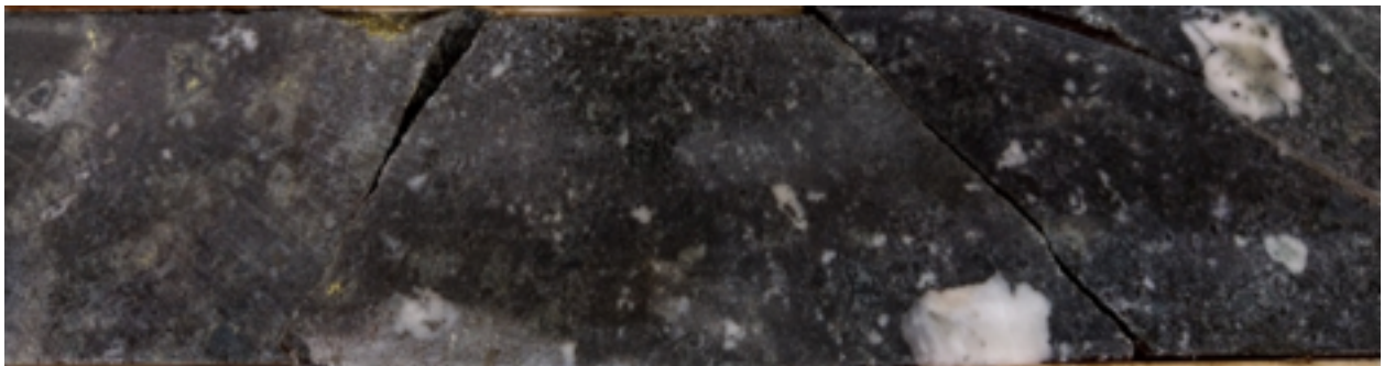
Figure 4: Dark norite breccia with disseminated pyrrhotite, chalcopyrite and probably re-melted felsic gneiss clasts. Width of the core: 4 cm. Photo: D. Klimentyeva
