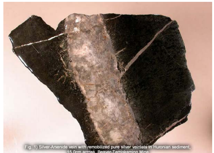
Figure 6: Polymetallic vein with remobilized Ag veinlets in Huronian sedimentary rock; ca. 15 cm across. Sample from Temiskaming mine. Photo from Joyce (2011).
