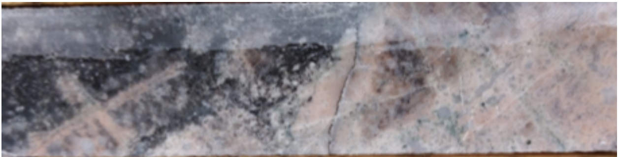
Figure 5: Clasts of veined granite in the norite breccia. Width of the core: 4 cm. Photo: D. Klimentyeva
