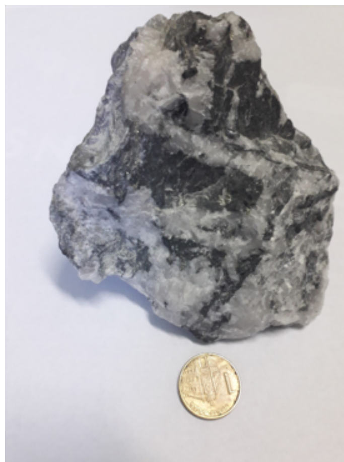
Figure 5: Sample from Lamaque mine, containing a quartz-tourmaline vein with pyrite and native gold. Photo: M.Velojic
