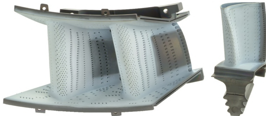
(b) Fully cooled high-pressure turbine vane and blade of the GP7000 equipped with thermal barrier coating [121]
