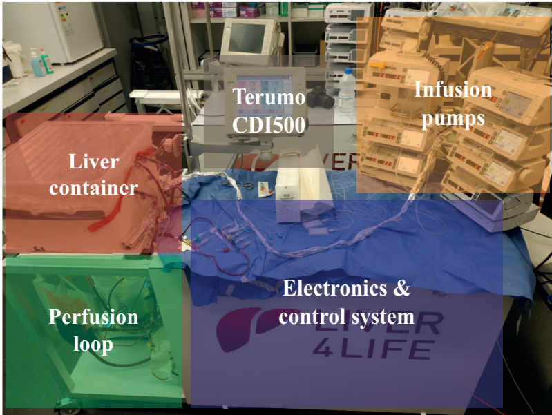
Figure 3.3: Image of the entire machine with liver container, perfusion loop, electronics & control system, Terumo CDI500 and infusion pumps highlighted.
