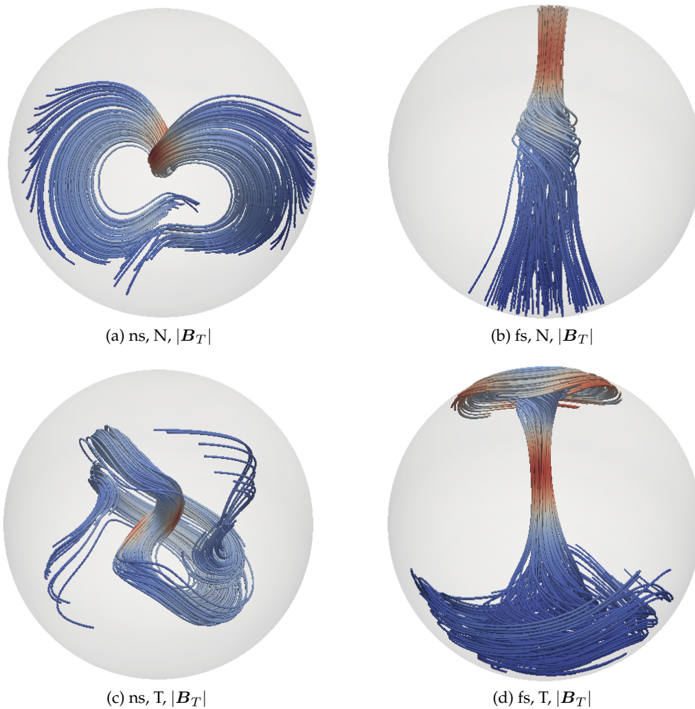
Figure 2: Field lines of eigenmodes \mathbf{B}_T corresponding to flows in Fig.1 with different magnetic boundary conditions. 'ns' and 'fs' denote no-slip and free-slip boundary conditions for the flow respectively; N and T stand for two magnetic boundary conditions used. The color scale gives the magnetic field magnitude (red is most intense).
