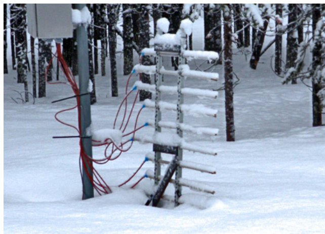
Figure 4. Snow temperature was measured with an array of horizontally oriented temperature sensors at the meteorological mast. Image modified after Lemmetyinen et al. (2013).
