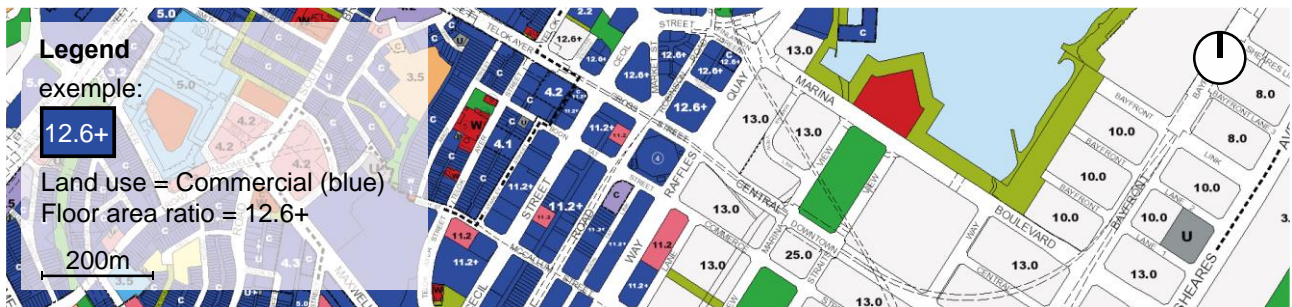
Figure 1. Density and land use control in an exemplary master plan (Urban Redevelopment Authority, 2014).
