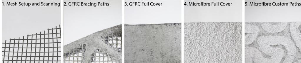
Figure 9 Robotic AeroCrete (RAC) spraying steps.
