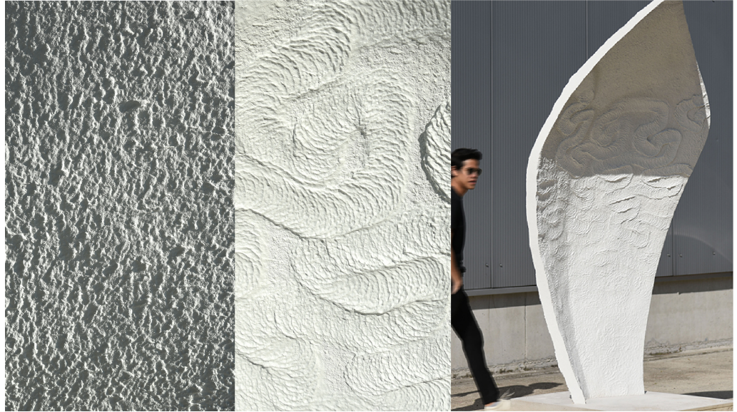
Figure 15 Left, Centre: Process inherent surface texture on front and back sides. Right: Final slender reinforced concrete Prototype.
