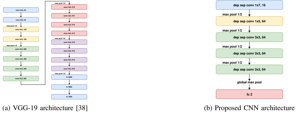
Fig. 4: CNN architectures: The annotations "dep sep conv 1 \times 7, 16 " represent a depthwise separable convolutional layer with a 1 \times 7 convolutional filter and 16 channels and "fc 2" a fully connected layer with two outputs, respectively. Max pooling is abbreviated as "max pool".
