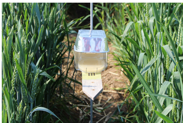
Fig. 2. Spore traps with Fusarium selective medium placed between two adjacent wheat varieties and adjusted to the same height as the flowering heads.
