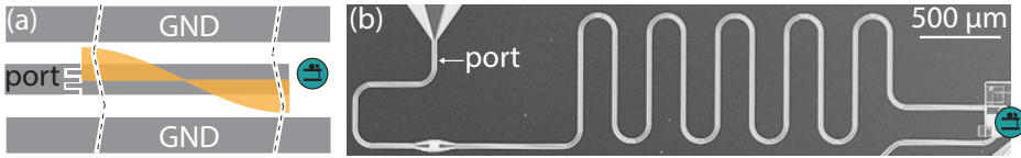
Figure 4.4 50\Omega resonator schematic and picture. (a) Schematic illustration of a coplanar waveguide \lambda/2 resonator that is capacitively coupled to a microwave port on one side and a qubit on the other side. (b) False-colored optical micrograph of the resonator from (a) that is fabricated from Al (dark gray) on top of GaAs (white).
