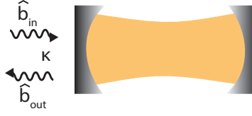
Figure 4.2 Cavity input-output model. Schematic illustration of a single-sided cavity that is coupled to input (in) and output (out) fields represented by the operators \hat{b}_{\text{in,out}} at coupling rate \kappa .
