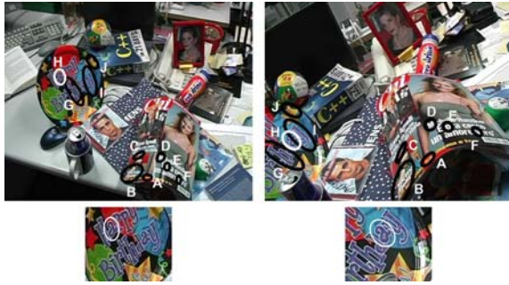
Figure 12. Felix scene. Top: 9 Matches. Bottom: Close-up on match H; the ‘a’ of ‘Happy’ is mismatched to ‘Birthday’. The GAM constructor successfully finds the two groups (dish, magazine) and isolates the mismatch in a third, singleton one.
