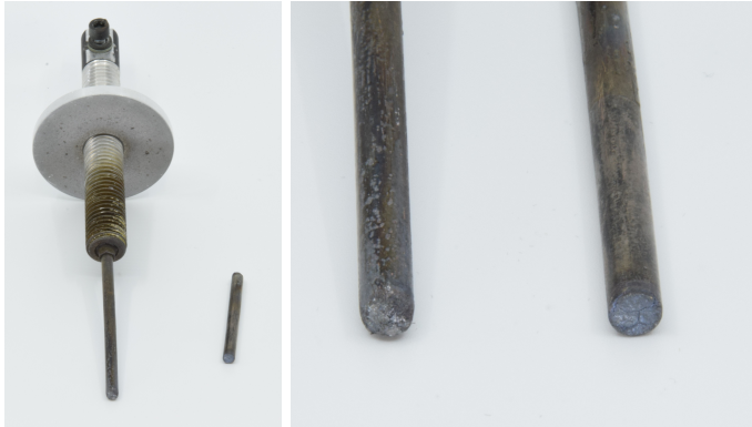
Figure 4.12: Overview (left) and closeup (right) of the 5 mm WCu contact pins. The downstream pin (left in both pictures) was always the anode. The initially cylindrical tip erodes into a convex tip. Additionally, many brighter spots can be seen on the side of the pin, these were created when the arc root was blown downstream along the side of the pin, as shown in figure 4.20. The upstream pin was always cathode, and showed different erosion. The tip became concave, and cracks formed at the surface.
