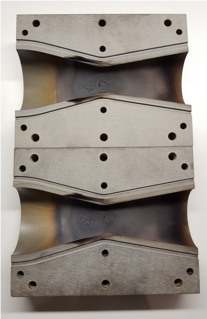
Figure 5.11: Ablation resistant nozzles after experiments. in contrast to homogeneous ablation in PMMA, the surface of S5000 material chars and cracks, until pieces break of.
