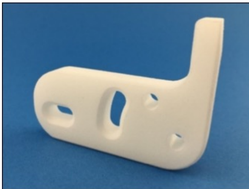
Fig. 3.1: Customer specific lug variant, manufactured in laser sintered PA12.
