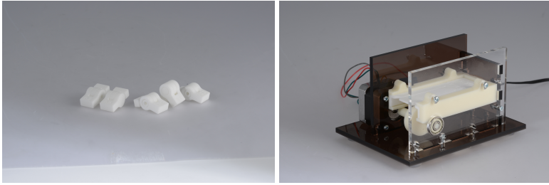
Fig. 4.5: On the left several hinges manufactured with different parameters for the purpose of feature testing. On the right, a low fidelity test bench for the feature testing of a snap fit durability.
