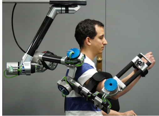
Fig. 1. Exoskeleton arm of ANYexo with a user.
