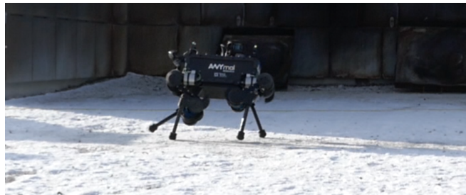
Fig. 1. ANYmal can walk blindly over ice and handle slipping contacts. A probabilistic slippage estimator triggers impedance control and friction modulation to stiffen the motion.
