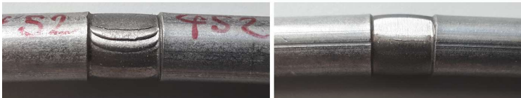
Figure 56: Misformed workpiece surfaces due to slippage
