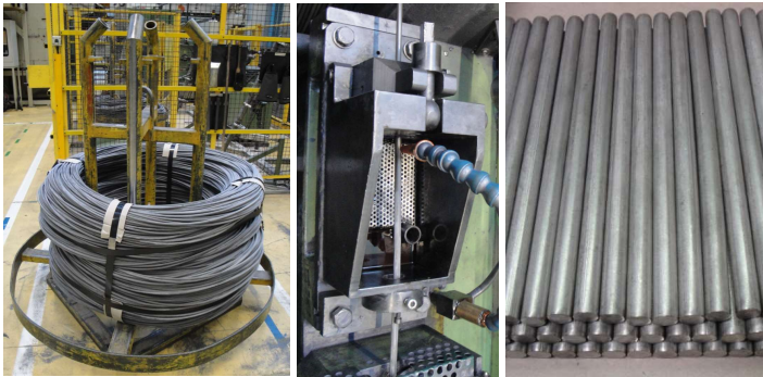
Figure 46: Left: Raw material delivered as wire coils before preparation, Middle: Wiredrawing, Right: Wiredrawn billets after preparation
