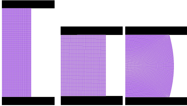
Figure 25: Left: Undeformed compressive probe, middle: Ideal deformation, no friction, right: deformed probe with friction
