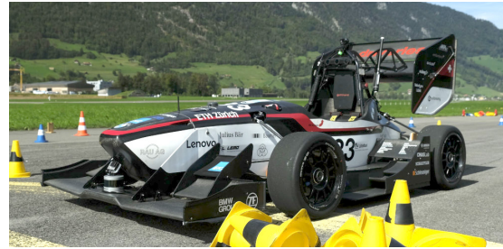
Fig. 1: gotthard is a driverless electric 4WD race car.
