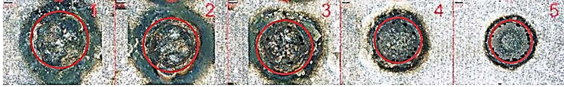
Fig. 3-19: Drilling tests with a different pulse duration from left to right: 5 \mu\text{s} ; 3 \mu\text{s} ; 2 \mu\text{s} ; 1 \mu\text{s} ; 0.6 \mu\text{s} ; U_{\text{open}} = 100 \text{ V} and polarity is positive in all experiments. The red circles indicate the border of the holes.
