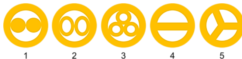
Fig. 2-6: The multi-channel electrodes configuration comparison [22, 87, 88]. Type 1 is used for flow simulation, this type is recommended by GF Machining Solutions, Agie Charmilles SA machine tool manufacturer for Drill 300.
