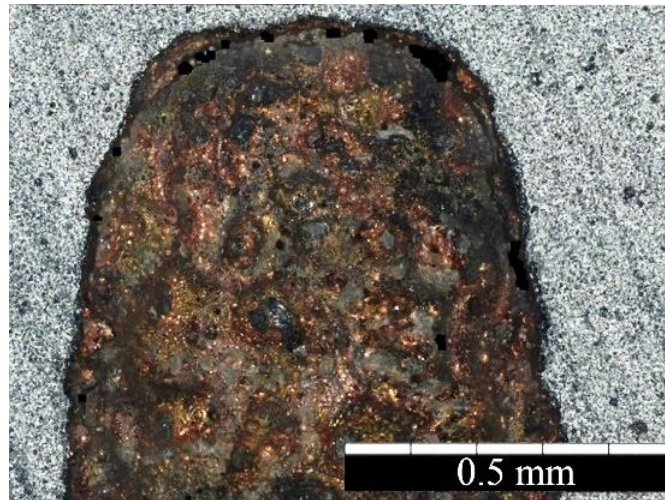
Fig. 3-34: Longitudinal section of an EDM drilled hole in SiC, using deionized water as a dielectric, solidified copper (red areas) are found on the machined surface.
