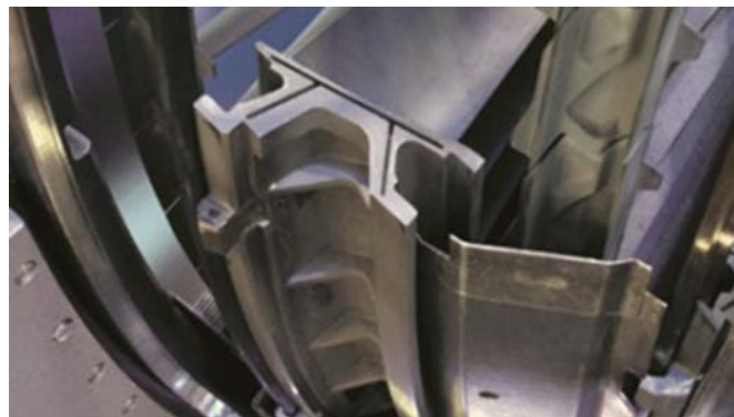
Fig. 2-4: Seal slot with a complex shape in nozzle guide vanes [52].
