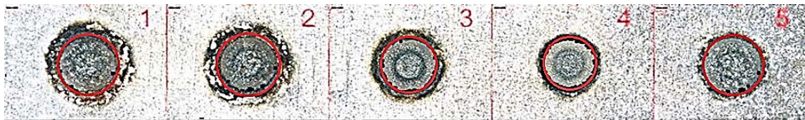
Fig. 3-21: Drilling tests with a different ignition voltage from left to right: 120 V; 100 V; 80 V; 60 V; 50 V; T_{\text{on}} = 1 \mu\text{s} and polarity is positive in all experiments. The red circles indicate the border of the holes.
