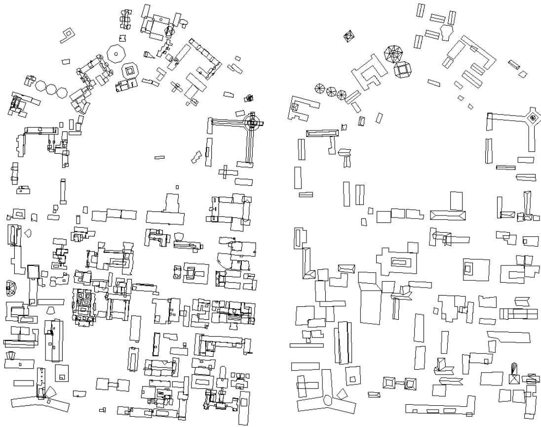
Figure 6. Buildings of University of Melbourne campus reconstructed from 1:15,000 aerial images (left) and from stereo Ikonos imagery (right). To simplify visualisation, first points and first lines have been omitted in the left figure.
