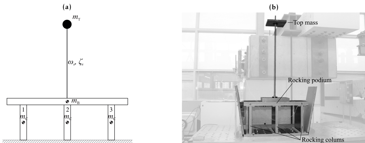
Figure 6.8: Experimental testing of rocking podium structures: (a) Dynamic model; (b) Experimental setup (1 st attempt).
