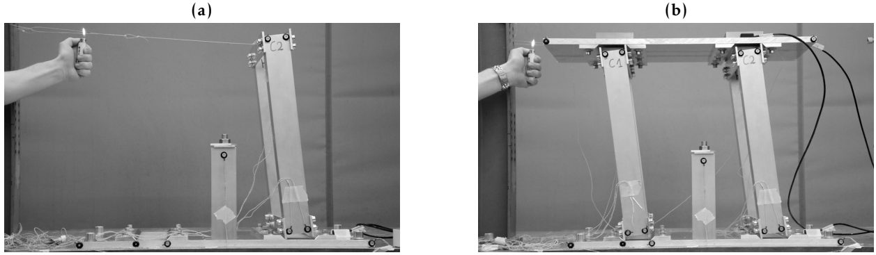
Figure 6.11: Calibration tests of sub assemblies: (a) Rocking column; (b) Rocking frame.
