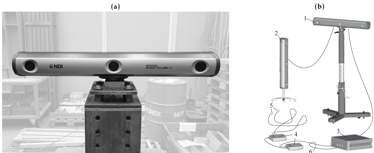
Figure 6.4: NDI, Optotrak Certus HD [144]: (a) Primary position sensor (No. 1); (b) Laboratory setup.
