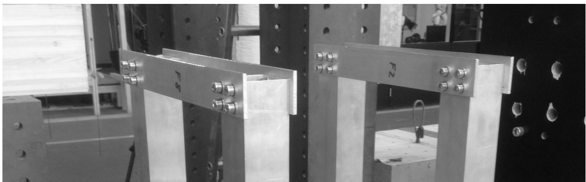
Figure 6.19: Carved edges of the rocking column.
