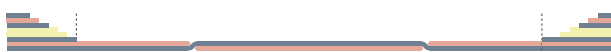
Fig. 8. Stacking sequence for one complete corrugation period. Dashed lines indicate transition to non-morphing parts of the design. For better visualization, the ratio between length and thickness is not to scale.
