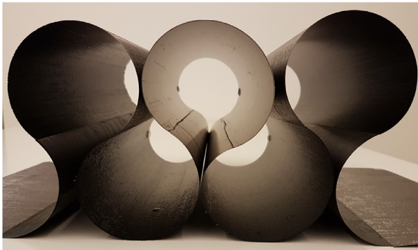
Fig. 24. Demonstrator laminate after laying process.
