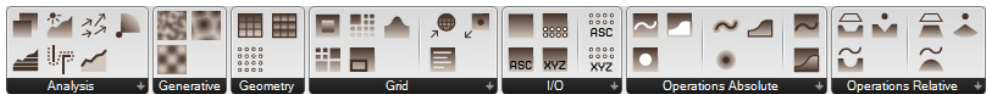
Fig. 1: Docofossor's toolbar in the visual scripting environment Grasshopper for Rhinoceros. Functions include the Absolute and Relative cut and fill operations, analysis tools, BRep construction, DTM import and export, and various grid operations.
