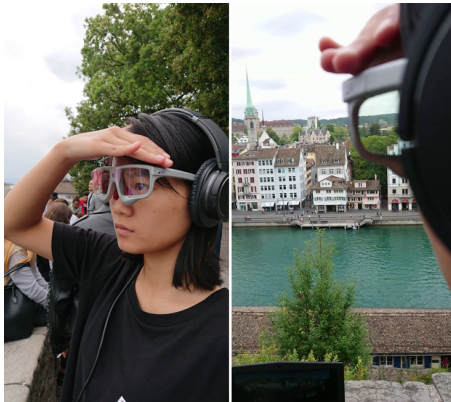
Figure 1: Gaze-based interaction with a city panorama. The system provides audio information about the buildings the tourist looks at [18].
