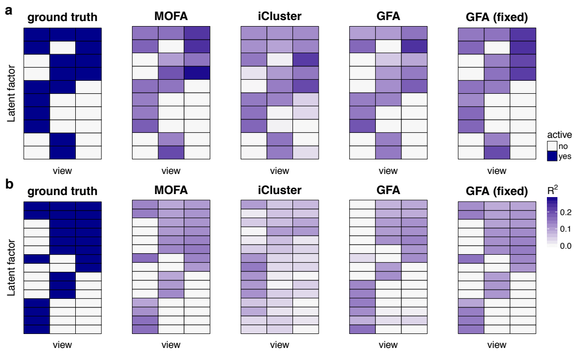
Figure 4.A.5: Assessment of MOFA, iCluster and GFA in terms of recovering the pattern of factor activity across views. Data were simulated using a Gaussian likelihood based on the true activity pattern of factors per view displayed on the left. (a) Number of true underlying factors K = 10 . (b) Number of true underlying factors K = 15 . In both cases, MOFA and GFA were trained starting with K = 25 factors whereas for iCluster and GFA (fixed) the true number of factors was used. Shown is the fraction of variance explained for each factor and view.
