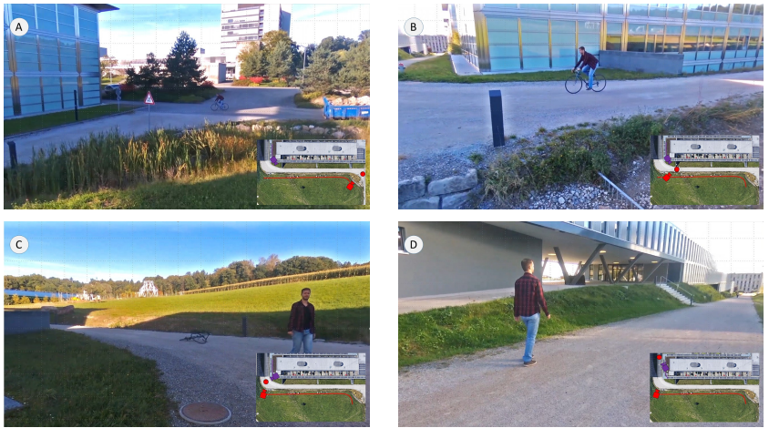
Figure 6.9.: Figures A - D: Multi-view, single-person shot outdoors. A+B: A person rides a bike along a street and is filmed by camera 1 (red). C+D: Person gets of the bike, switch to camera 2 (purple). camera 1 goes out of view of camera 2.
