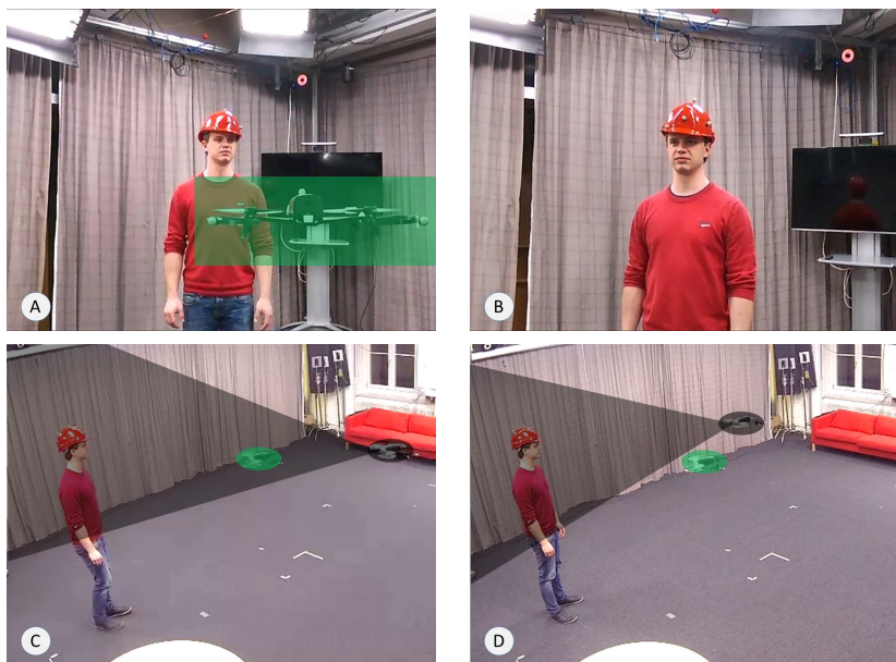
Figure 6.6.: Influence of penalizing mutual visibility. A and C: single subject is filmed by two drones simultaneously, the first drone (green) is in the field of view of the second drone. B and D: Enabling the mutual visibility cost triggers re-planning of trajectory resulting in unobstructed view with correctly framed subject.
