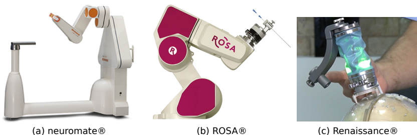
Figure 2.1 : Robot arms used in neurosurgery. (a) neuromate ® stereotactic robot from Renishaw (Gloucestershire, UK). (b) ROSA ® robot from Medtech (France). (c) Renaissance ® guidance system from Mazor Robotics (Caesarea, Israel).
