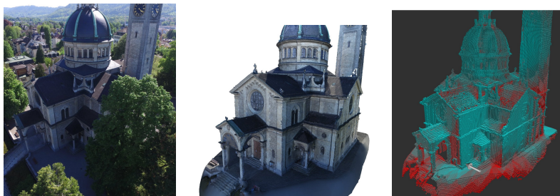
Figure 1.2: Shown on the left is a color image of a church. The middle pane shows a rendering of a mesh representation and the right pane shows a rendering of the occupancy map representation.
