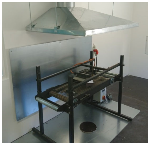
Fig. 4: Pyrolysis machine: (1) Energy source carrier, (2) Propane connection, (3) CO 2 line, (4) Gas burner, (5) Propane gas line, (6) Pick-up reel, (7) Slide rails, (8) Drive gear, (9) Conveyor belt frame, (10) Conveyor belt tensioner, (11) Drive gear, (12) Nitrogen connection, (13) Base frame, (14) Motor, (15) Control cabinet, (16) Rotary feet.
